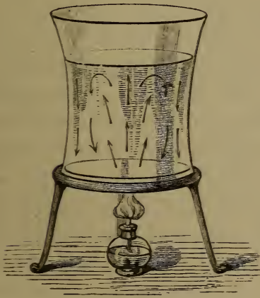
FIG. 46.—Currents in water by heat.
